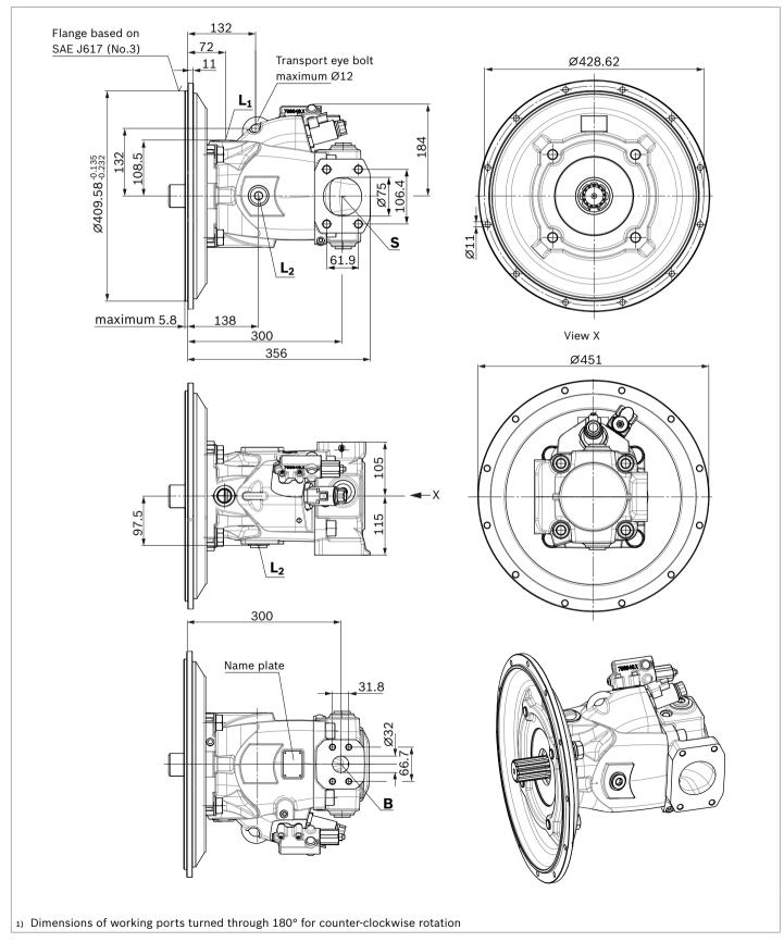
EP4DR – Electric-proportional control with pressure controller, clockwise rotation, mounting flange G3 (SAE J617)<sup>1)</sup>
