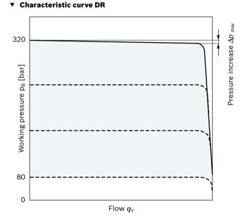
Characteristic curve valid for  $n_1 = 1500$  rpm and  $t_{fluid} = 50$  °C.
