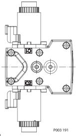
A serviceable 125  $\mu$ m screen is located in the supply line immediately before the control porting spool.
